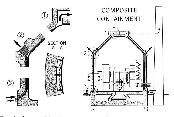
Figure 2: Separation of the cooling air stream from the filtered air stream
