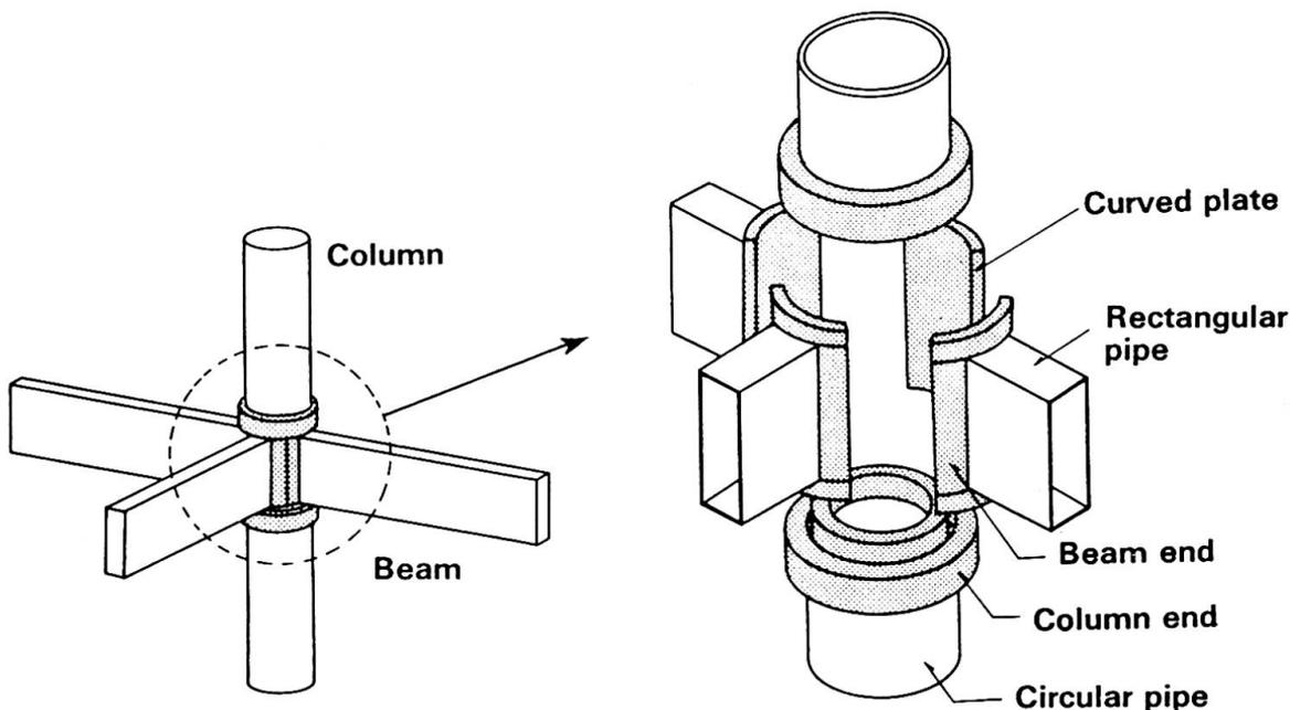
Fig. 3 Column-to-beam joint
