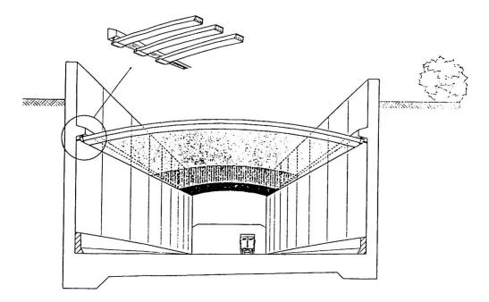
fig. 9: Perspective view of a tunnel daylight screen
