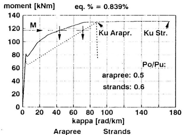
fig. 2: moment-rotation curves of the slabs of fig.1
