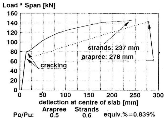
fig. 1: deflection at mid span of a slab prestressed with steel and with Arapree
