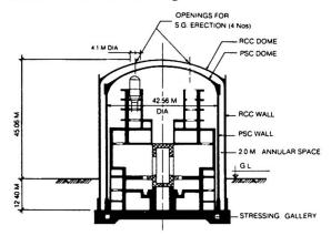
Fig.6 Section of Kaiga Containment
