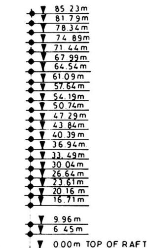
Fig.4 Mass lumping at floor levels for Dynamic Analysis
