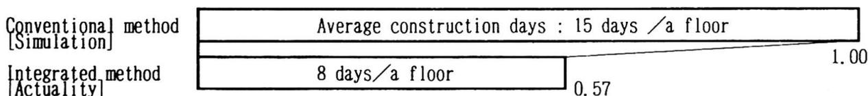
Fig. 8 The comparison of the construction speed
