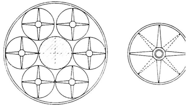
**Fig. 3** While smaller units can operate with a single wind turbine, larger power plants would work better with several turbines. During operation, automatically controlled setting gears adjust the blades to their optimal face-impact angle.
