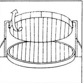
The front membrane is then deformed to a paraboloid by applying air pressure between the membrane and the ground and subsequently fixed to the ring.
