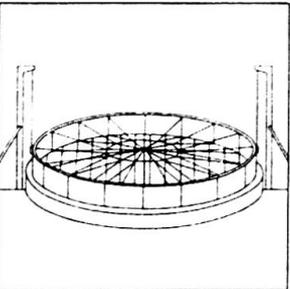
After fixing the rear membrane to the ring the concentrator is turned over.
