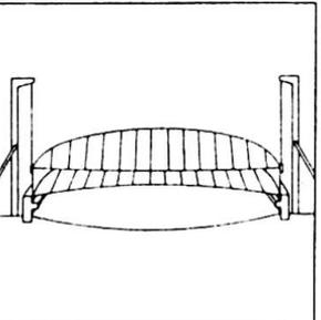
Now the air can be extracted from the concentrator housing thus created; with a partial vacuum between them the membrane surfaces will also withstand high wind loads.
