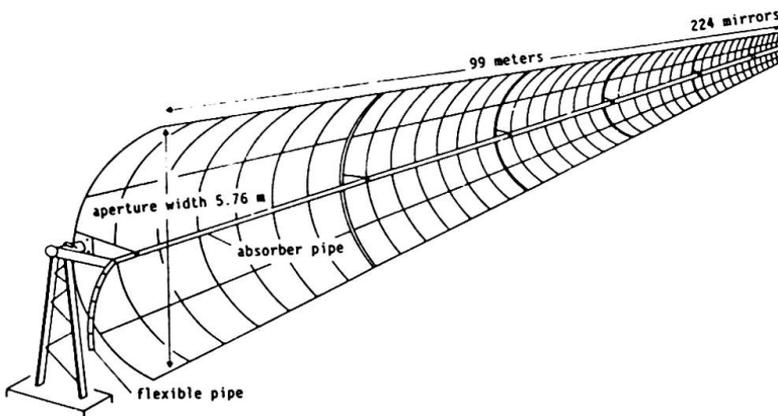
**Fig. 6** Sketch of the LS-3-Collectors as built by Luz International Ltd. and Flachglas-Solartechnik GmbH
