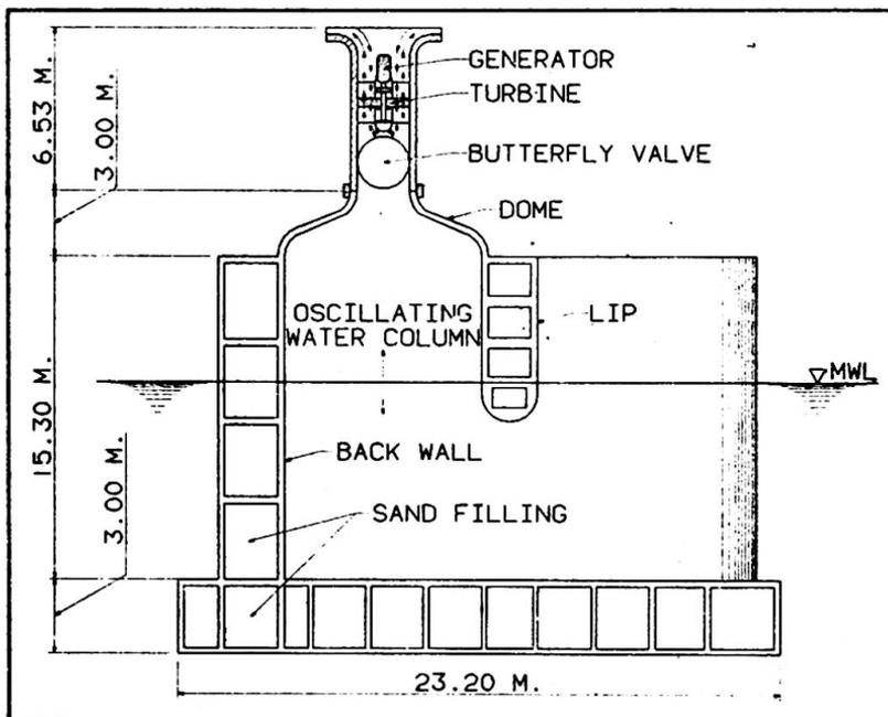
**Fig.3** Experimental wave energy generator offshore Tamil Nadu
