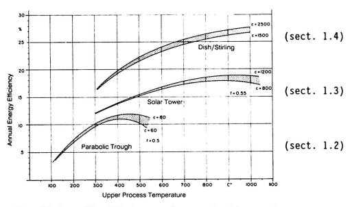
Fig. 11 Overall efficiency of concentrating systems
