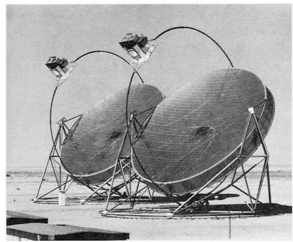
Fig. 9 Two 50 kWe concentrators in Riyadh
