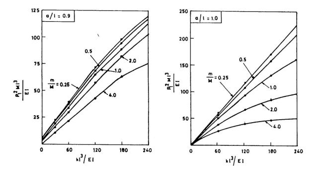
FIG.3 VARIATION OF FIRST BENDING FREQUENCY
