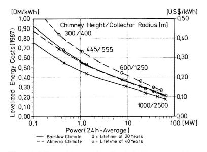
Fig. 5 Solar chimneys's electricity generating costs in relation to mean installed power
