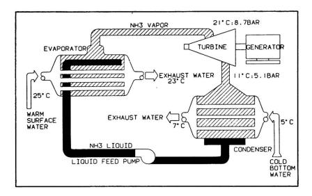
Fig.1 Scheme of closed cycle OTEC plant
