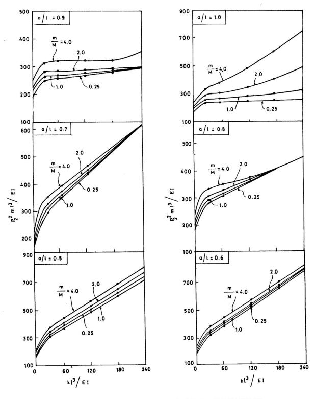
FIG-4 VARIATION OF SECOND BENDING FREQUENCY
