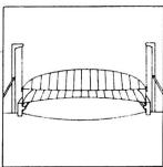
Now the air can be extracted from the concentrator housing thus created; with a partial vacuum between them the membrane surfaces will also withstand high wind loads.
