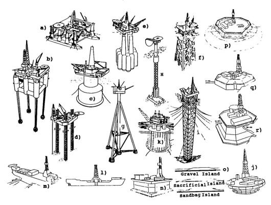
Fig. 1 Selected offshore structures: a) semi-submersible platform; b) tension leg platform; c) buoytype; d) jack-up; e)gravity platform; f) jacket-type; g) steel tripod; h) articulated tower; i) guyed tower; j) steel caisson; k) GBS platform; l) drillship; m) single steel drilling caisson; n - r) arctic structures /1, 10/.
