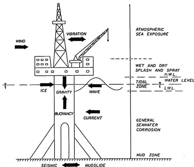
Fig. 2 Major platform loads and corrosion zones.
