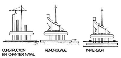
Fig. 12 Construction phases.
