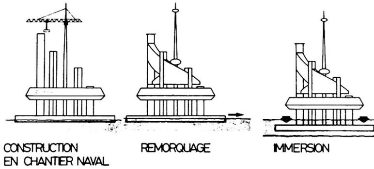
Fig. 12 Construction phases.
