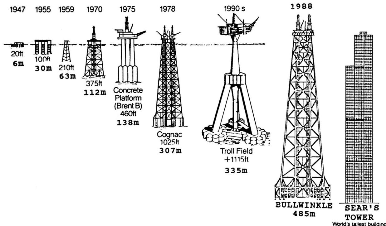
Fig. 3 Evolution of offshore platform design /4/.
