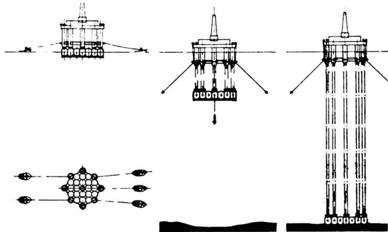
Fig. 24 Diagram of platform installation on the site.
