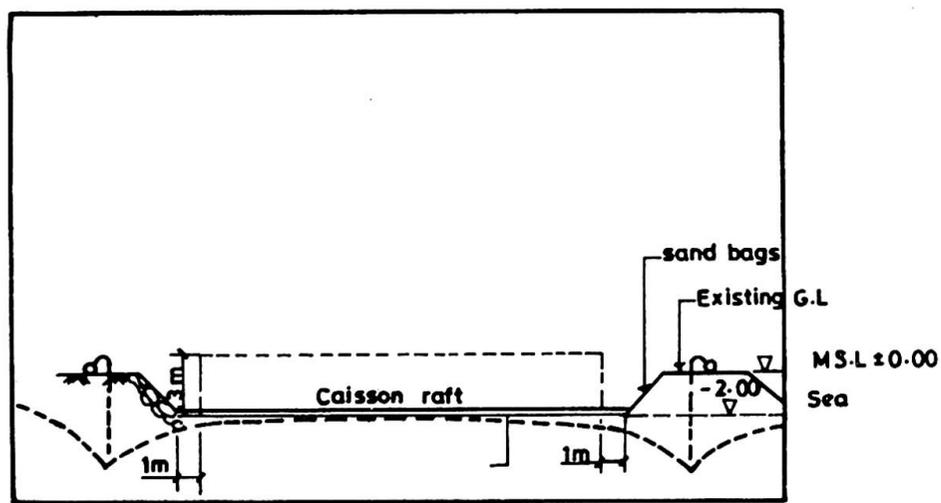
Fig. 3.a Construction of bottom box and bund
