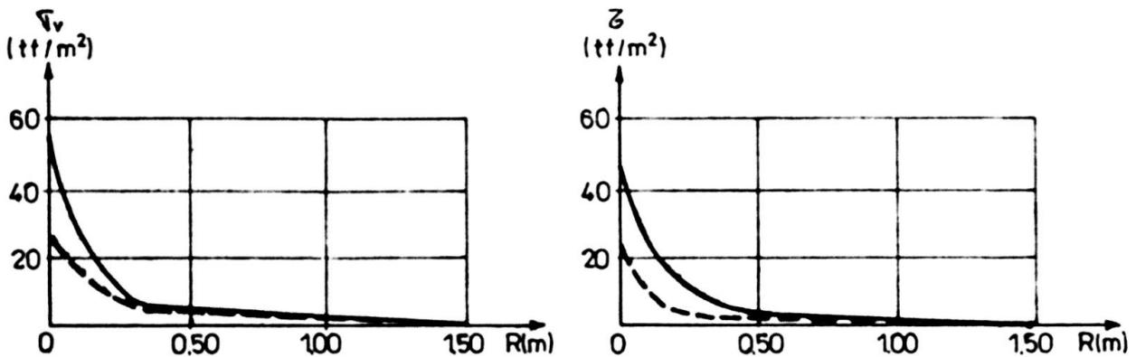
Fig.5 Diagramme of normal and tanqential unitary efforts at the level of the contact area between bulb and prebulb
