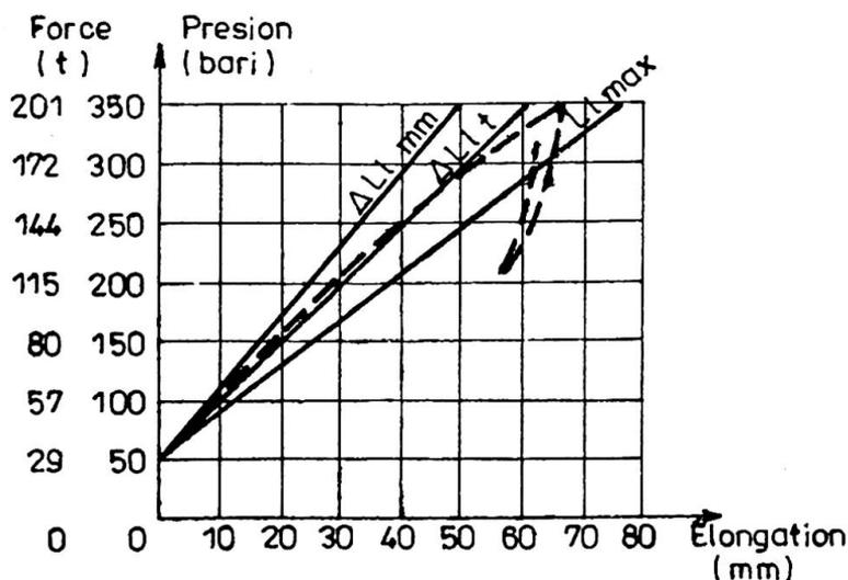
Fig.7 Diagramme of the tie-bar tensioning
