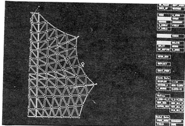
Figure 2 - Topology menu: adding link to boundary cable
