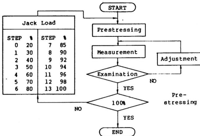
Fig.9 Flowchart of Prestressing and Measurement
