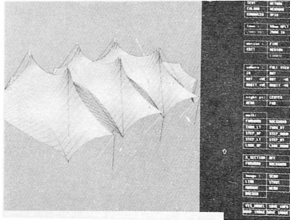
Figure 7 - Cutting pattern cloth display
