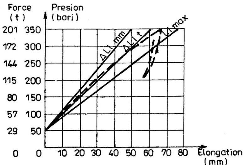
Fig.7 Diagramme of the tie-bar tensioning
