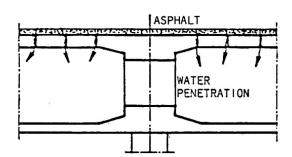
Fig.4 - BRIDGE DECK WITHOUT WATERPROOFING
