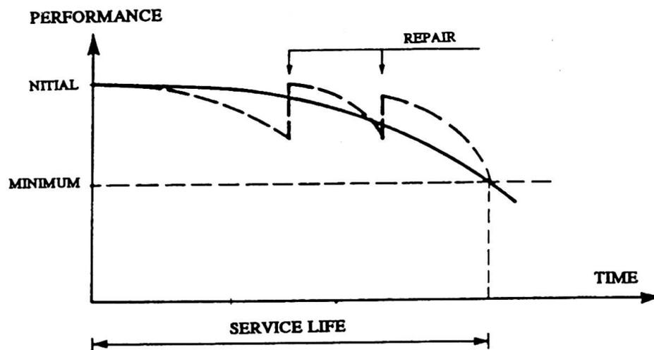
Fig. 1 Durability performance and service life of structures.
