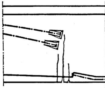
Fig. 14 - TENDONS ANCHORING
