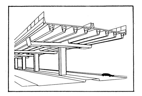
Fig.6 U-Beam Section
