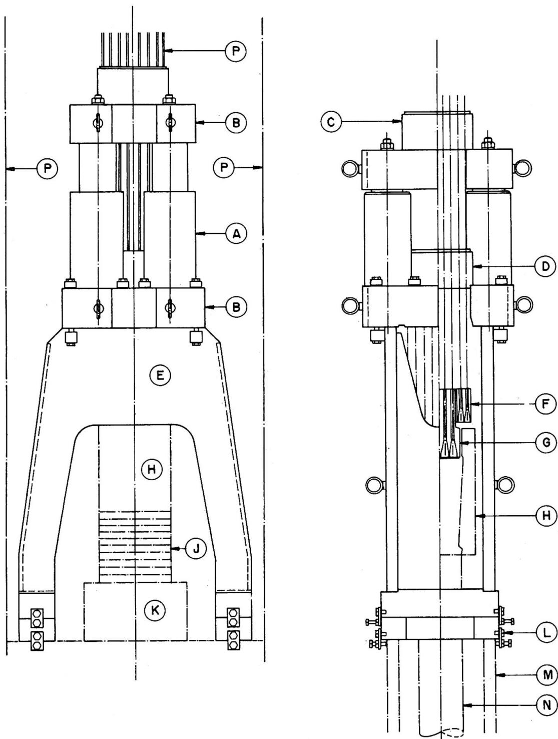
**Fig. 3 3F/Vemac 600 Tonne Cable Stressing System - Jack and Stool**
