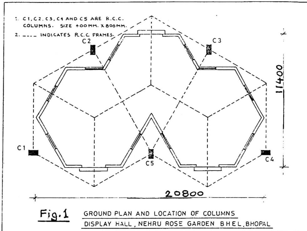
reinforced concrete with overall plan dimensions of 11400x20800mm. The entire roof structure rests on five RCC columns, each size 400x800 mm shows as  $C_1$  to  $C_5$  resting on rectangular RCC footings on soft rock with SBC of  $25 \text{ T/m}^2$ . It is 1500 mm below the ground level. A hinge of size 250x650 mm, length being 500mm is provided at 1000mm above the base of the footing to facilitate hinge action.
