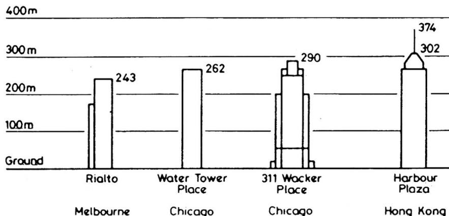
Fig. 1 - Tall buildings of concrete construction [7]
