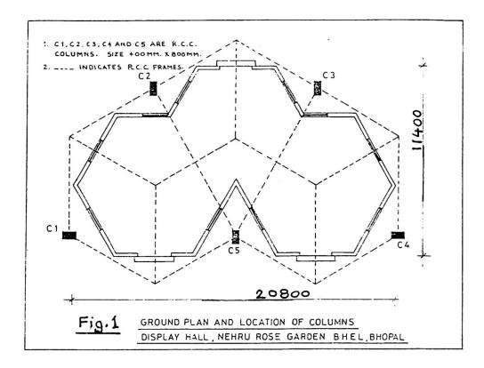
reinforced concrete with overall plan dimensions of  $11400 \times 20800 \, \mathrm{mm}$ . The entire roof structure rests on five RCC columns, each size  $400 \times 800 \, \mathrm{mm}$  shows as  $C_1$  to  $C_5$  resting on rectangular RCC footings on soft rock with SBC of 25 T/m². It is 1500 mm below the ground level. A hinge of size 250 x 650 mm, length being 500 mm is provided at 1000 mm above the base of the footing to facilitate hinge action
