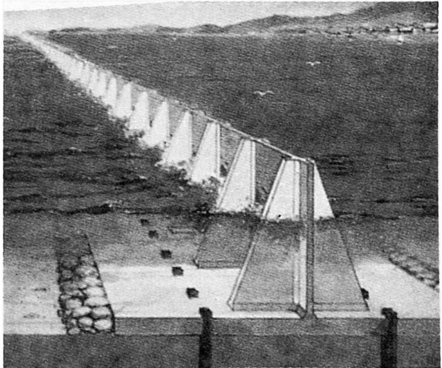
**Fig.3** Breakwater installed directly on soft seabed.
