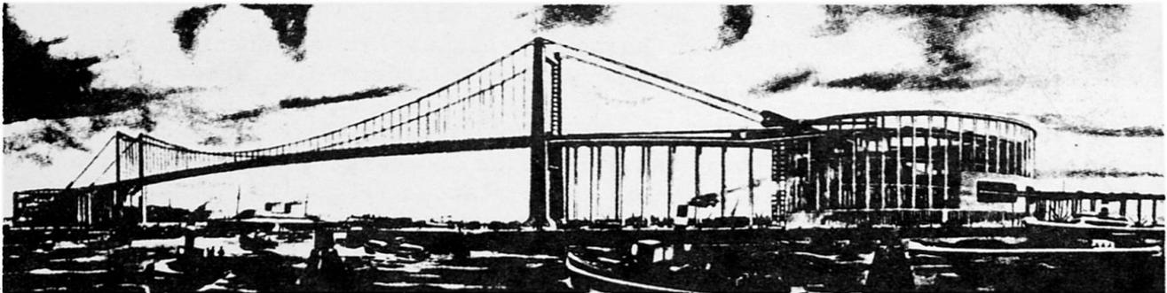
Fig.3 A bridge with spiralttype access structures as proposed for the Maastunnel in Rotterdam.
