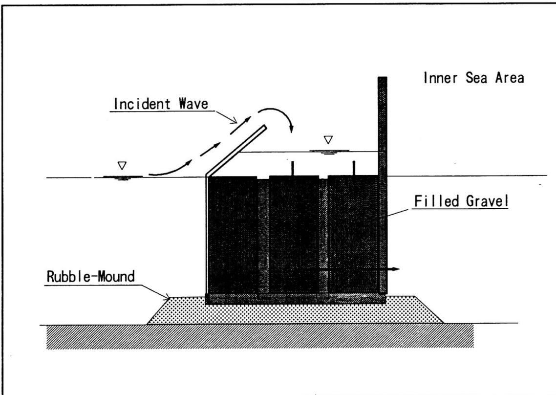
Fig. 12 Conceptual drawing of hybrid clean-up breakwater structure
