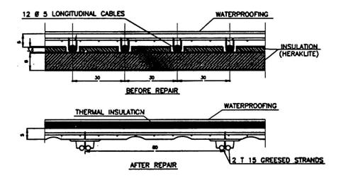
Fig.2 Section through shell
