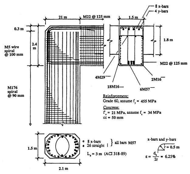
FIG 8. I-980, Bent #38 Reinforcement Details
