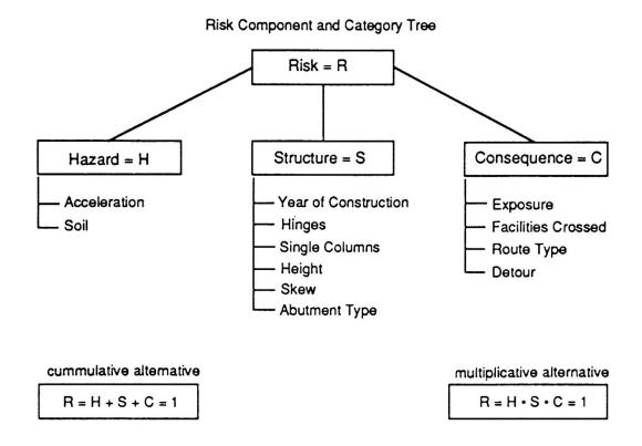
FIG 3. Seismic Risk Assessment Algorithm
