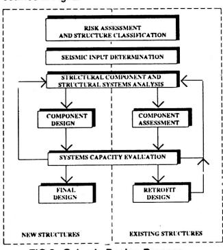
FIG 2. Seismic Design Process
