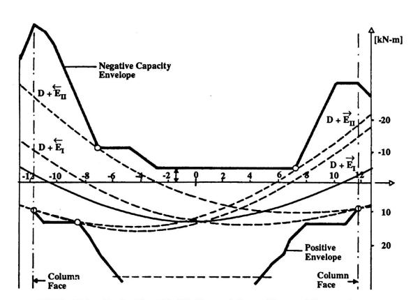
FIG 7. China Basin, Bent N<sub>1</sub>-35, Moment Capacities and Demand
