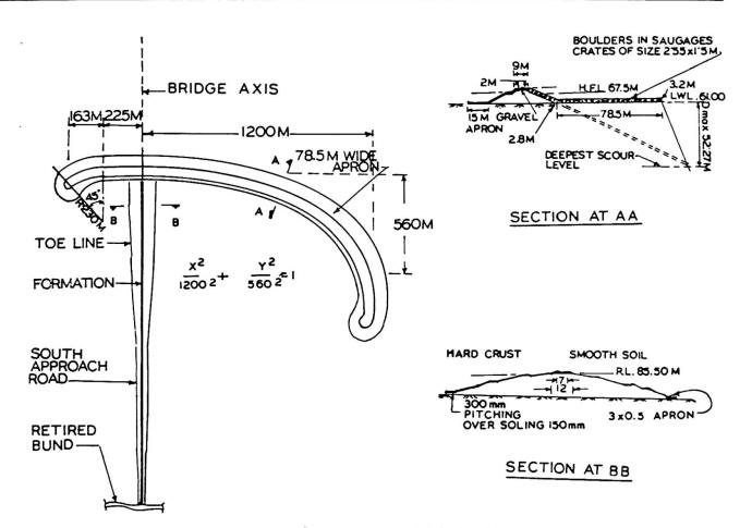
FIG. 5. GUIDE BUND DETAILS OF TEZPUR BRIDGE.
