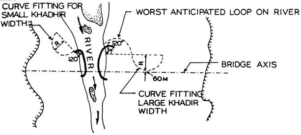
FIG. 6. DESIGN OF GUIDE BUND FROM LOOP CONSIDERATION
