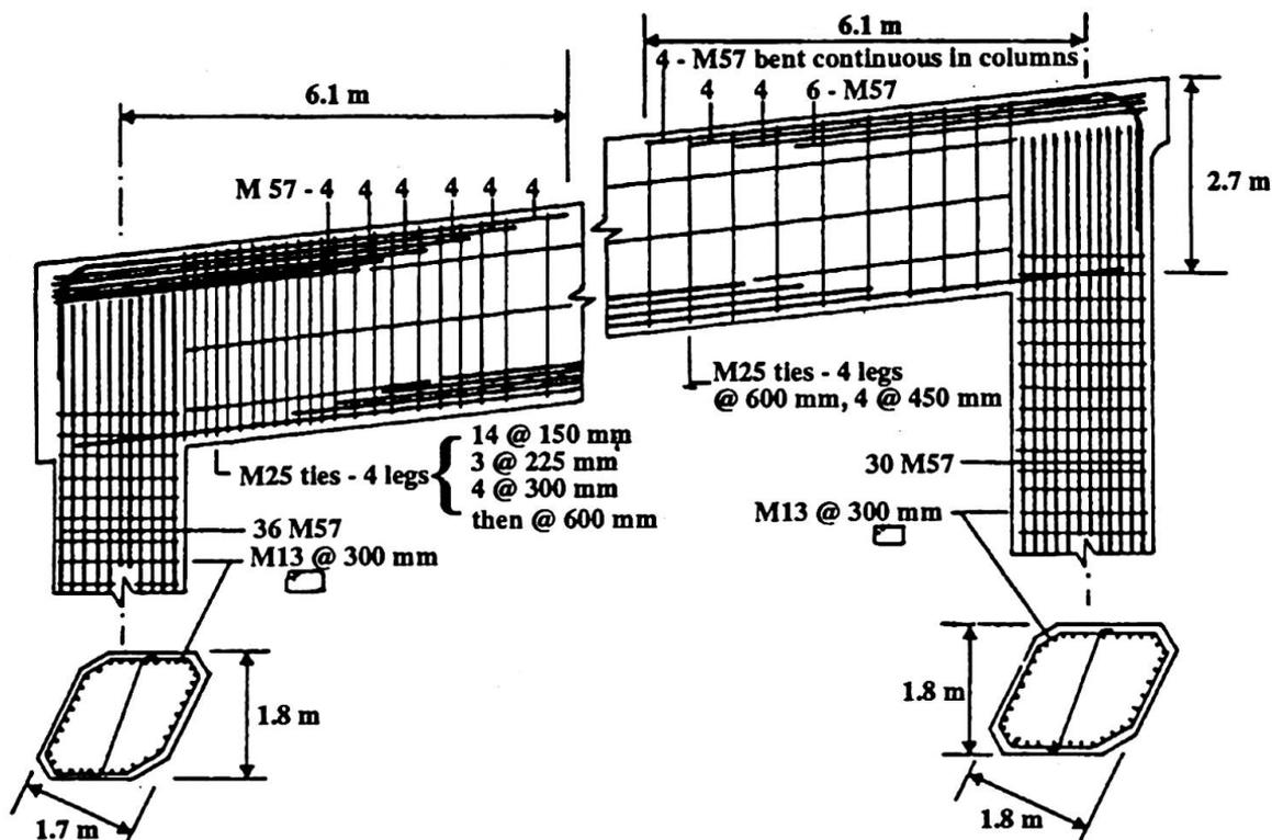
FIG 6. China Basin, Bent N<sub>1</sub>-35 Reinforcement
