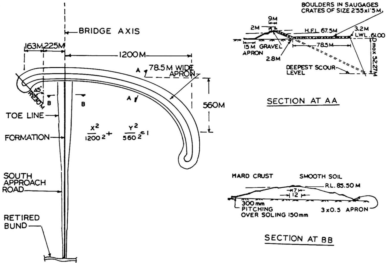
FIG. 5. GUIDE BUND DETAILS OF TEZPUR BRIDGE.
