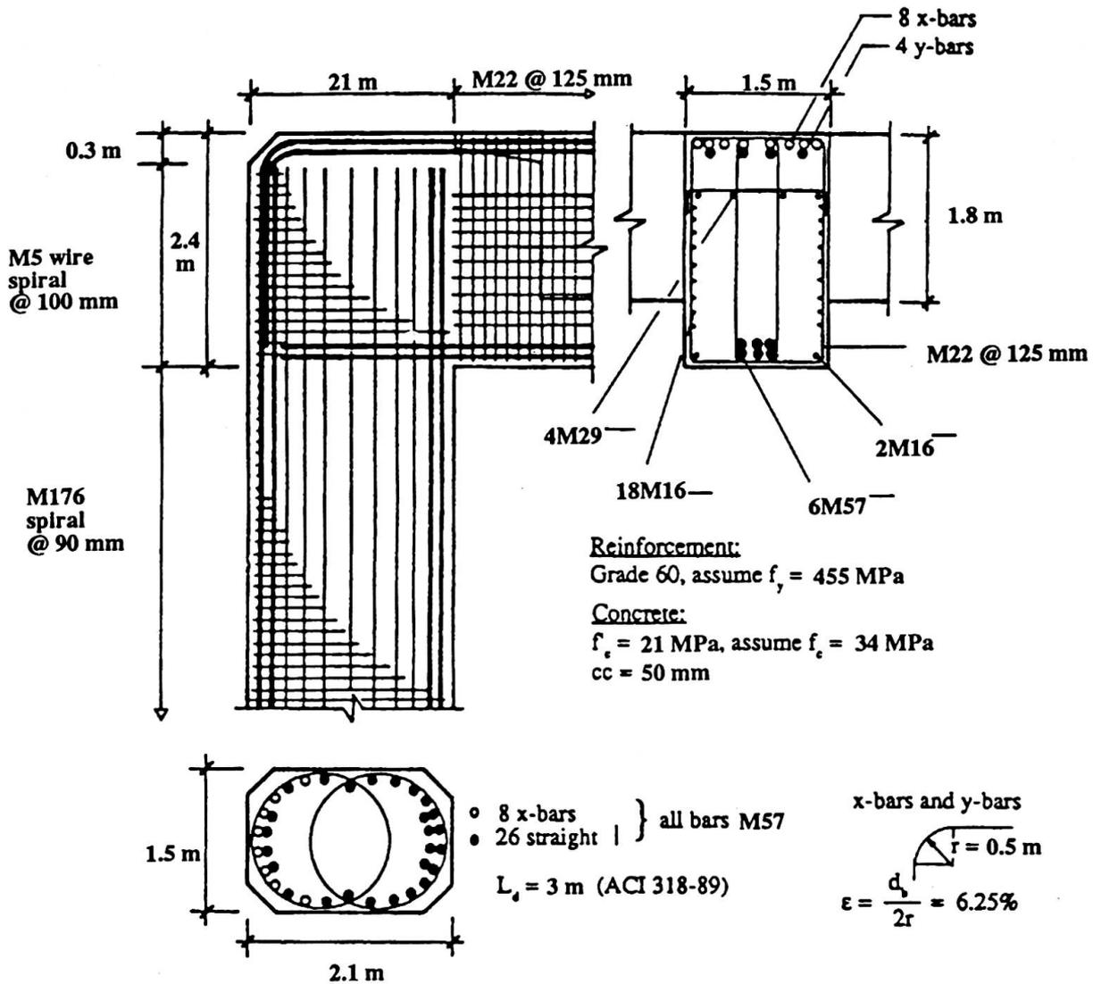
FIG 8. I-980, Bent #38 Reinforcement Details
