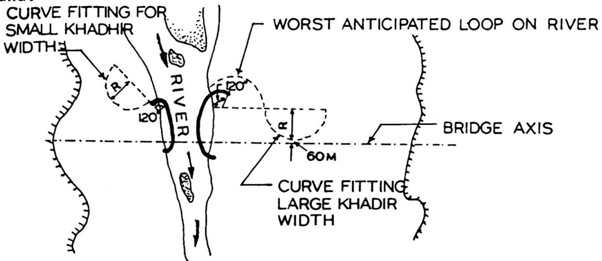
FIG. 6. DESIGN OF GUIDE BUND FROM LOOP CONSIDERATION
