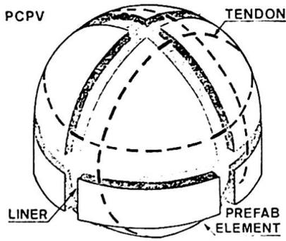
Fig. 1 Prestressed Concrete Pressure Vessel. Original concept after [3].
