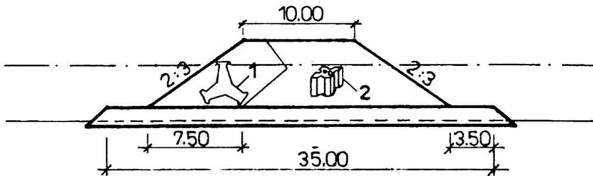
Fig.4 Breakwater-cross section
