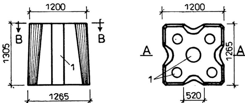
Fig.5 Concrete block (B=150 KN) acted biologically
