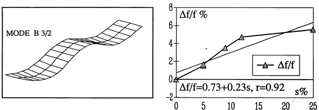
**Fig. 1** A bending mode for the prestressed concrete bridge and the relative difference in resonant frequency as a function of a damage index  $s$ , with regression-line and correlation coefficient  $r$ .
