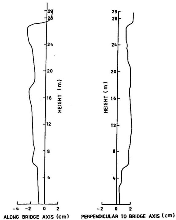
FIG. 2 (b) INITIAL PROFILE OF INCLINOMETER CASING
