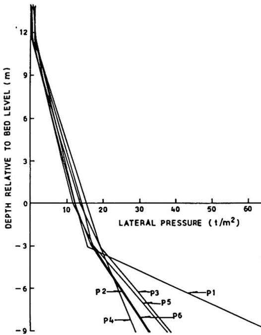
FIG. 2 (a) LATERAL PRESSURE VALUES OBTAINED FROM PRESSURE CELLS ( $t/m^2$ )
