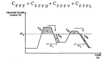
Fig. 1 Simplification proposed for the traffic flow curve versus time of the day
