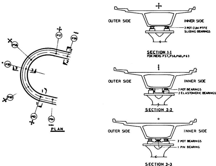
Fig. 3 Bearings for Loop Portion
