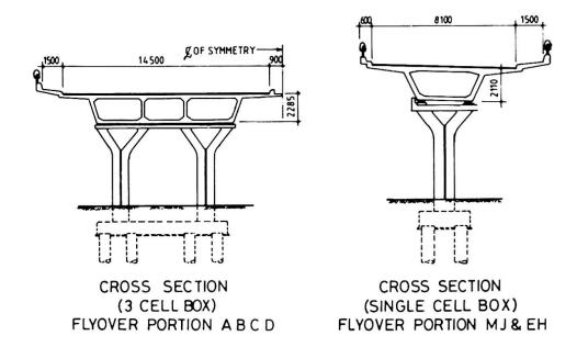
Fig. 2 Cross Section of Flyover portion
