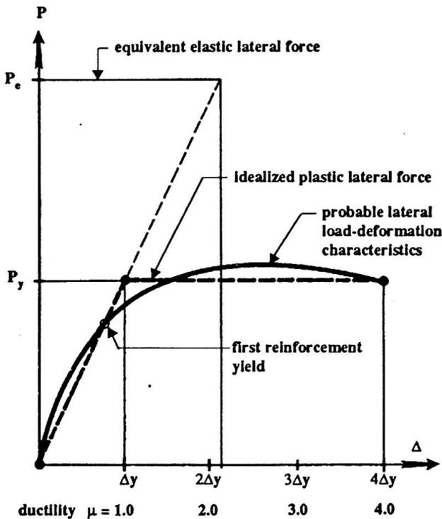
**FIG 4. Load Deflection Behavior and Equivalent Elastic Forces**
