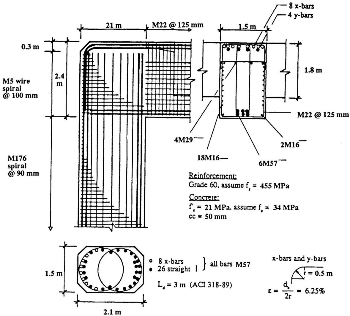
FIG 8. I-980, Bent #38 Reinforcement Details
