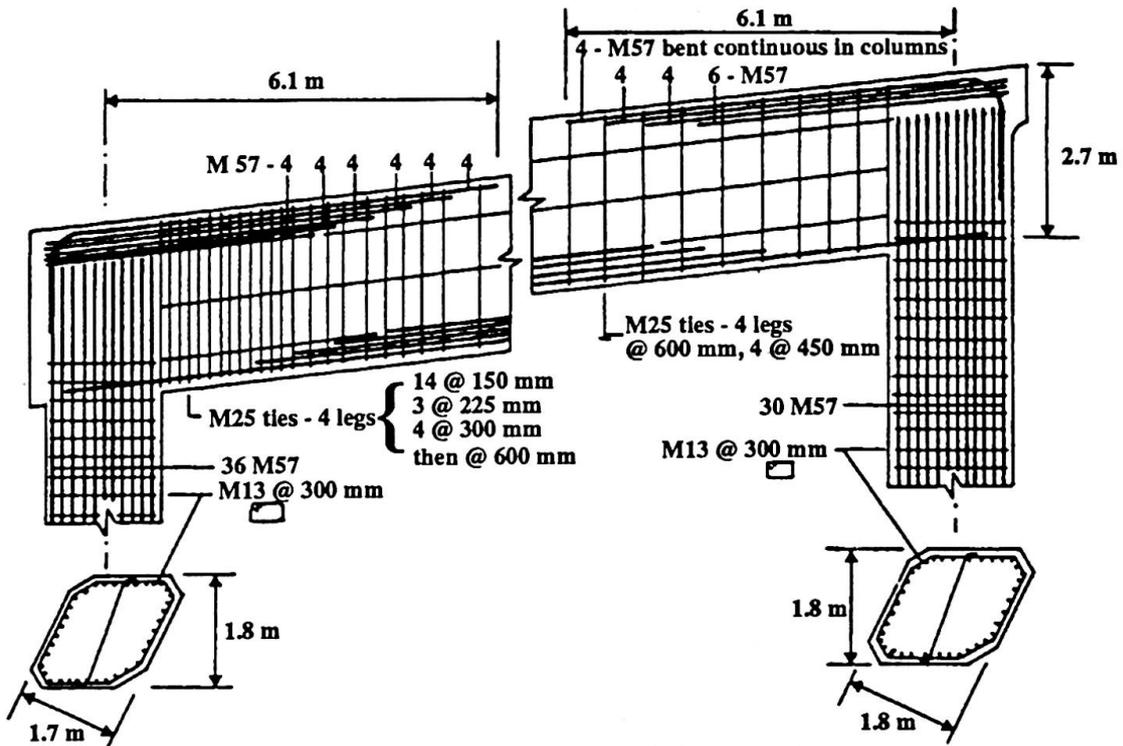
FIG 6. China Basin, Bent N<sub>1</sub>-35 Reinforcement
