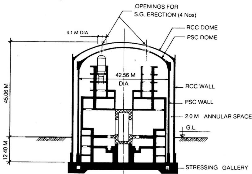
Fig.1 Cross Section - Kaiga Atomic Power Project
