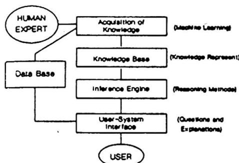
Figure 1. Typical Expert System Architecture
