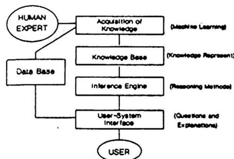
Figure 1. Typical Expert System Architecture
