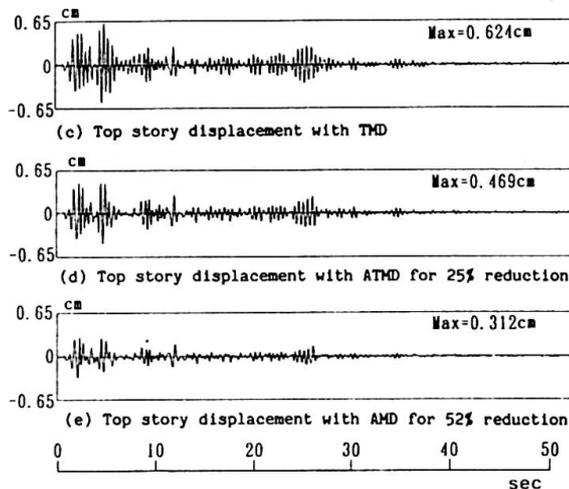
Fig.5 Active Control of the 4 Story Building Model
