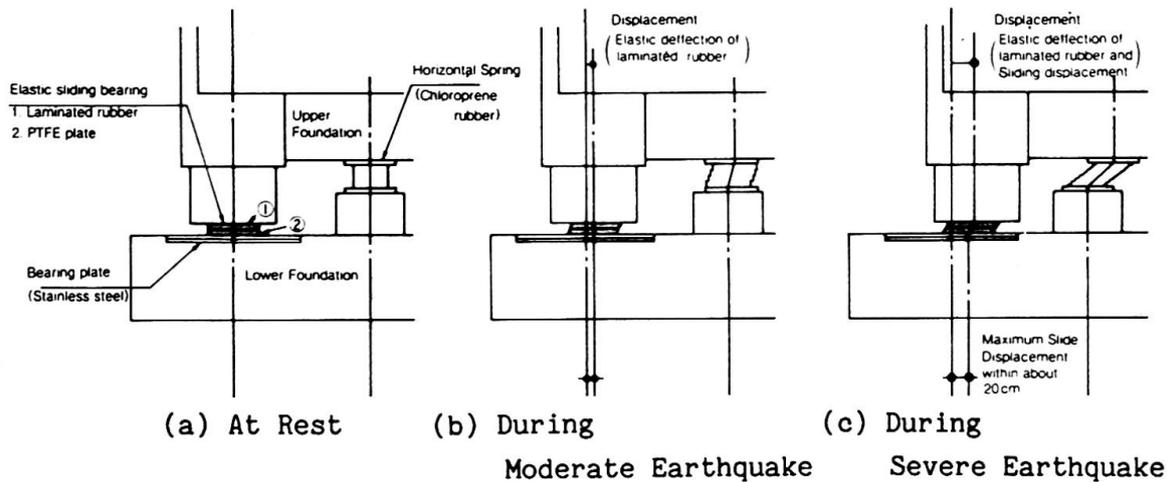
Fig.1 Composition and Isolation Mechanism of TASS System
