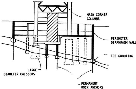
Figure 3: Schematic Section through Substructure and Foundation
