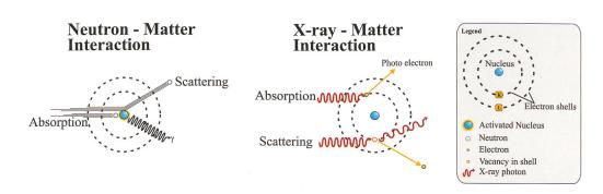
element can have strongly deviating properties. A deep knowledge of the materials behavior is needed to decide about the best experimental strategy. The cross-section data, which are values for the interaction probability with matter, are tabulated in specific data bases<sup>3</sup>.
