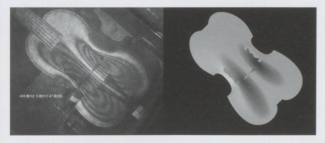
Figure 6::The first significant mode of vibration observed using ESPI (left) and simulation (right). Photo/graphics: IWK
