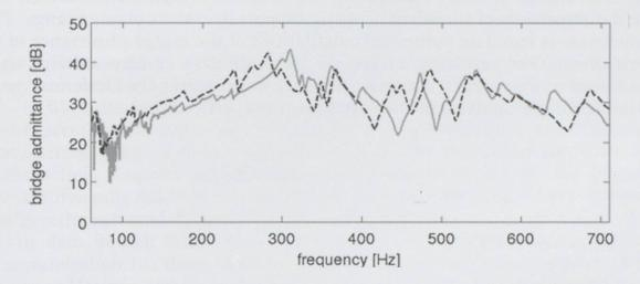
Figure 5: Bridge admittance measurements for two reconstructed instruments
