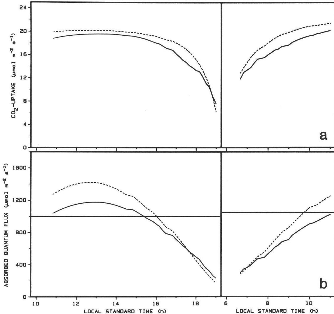
Fig. 8 a, b. Modeled diurnal courses of  $\text{CO}_2$ -uptake (a) and the weighted mean of absorbed quantum flux (b) per unit leaf area for the naturally curved lamina (—) of *Ficus carica* and a hypothetical flat leaf (---) with the same midrib orientation. The horizontal lines at 1000 and 1050  $\mu\text{mol m}^{-2} \text{s}^{-1}$  correspond to the saturating values of absorbed quantum flux in the afternoon and morning respectively.
