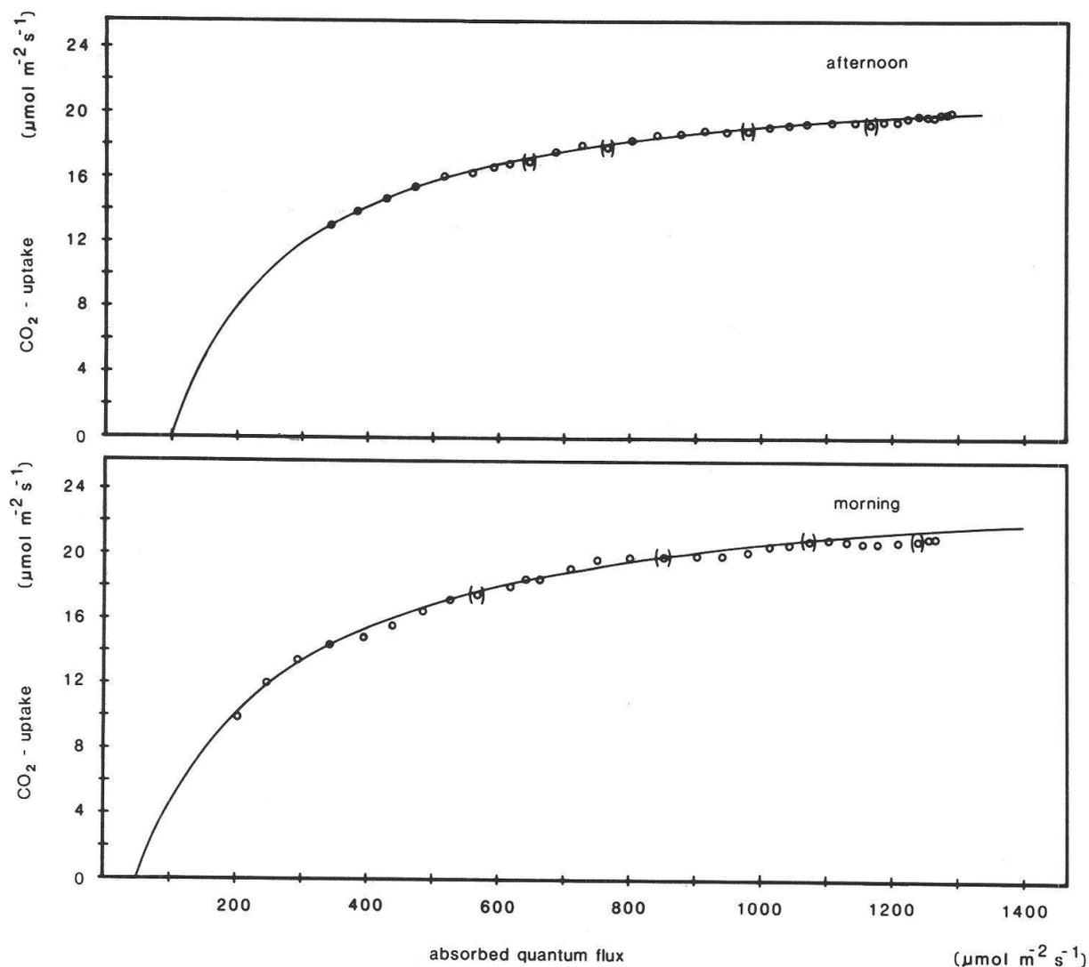
Fig. 3. Measured saturation curves (o) of CO<sub>2</sub>-uptake in the afternoon and morning of the *Ficus carica* leaf with the adjusted rectangular hyperbola (parameters in the afternoon:  $a=0.01190$ ,  $b=0.5998$ ,  $r=27.38$ ; parameters in the morning:  $a=0.005577$ ,  $b=0.1816$ ,  $r=7.103$ ).
