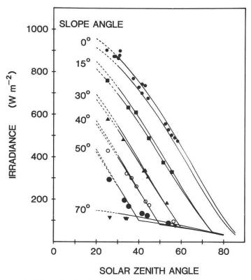
Fig. 4. Measured (symbols) and calculated (solid lines) global irradiation on planes with different slope angles in the sun's vertical (180° azimuthal difference to the sun) as a function of solar zenith angle. The calculation was performed for 15 km (lower solid lines) and 50 km (upper solid lines) sea-level meteorological ranges.
