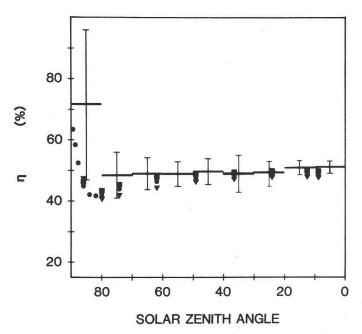
Fig. 5. Measured ratio  $\eta$  of PAR to global radiation (horizontal bars with standard deviation) as a function of solar zenith angle ranges (redrawn after Stanhill and Fuchs 1977) and corresponding values calculated for 12 km ( $\blacktriangledown$ ), 23 km ( $\bullet$ ) and 50 km ( $\blacksquare$ ) sea-level meteorological range.
