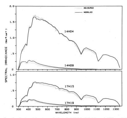
Fig. 2. Measured and calculated horizontal global (14h04, 17h15) and diffuse (14h09, 17h19) spectral irradiances on February 10, 1987 near Nieuwoudtville (Cp., Rep. South Africa). Time: local standard time.
