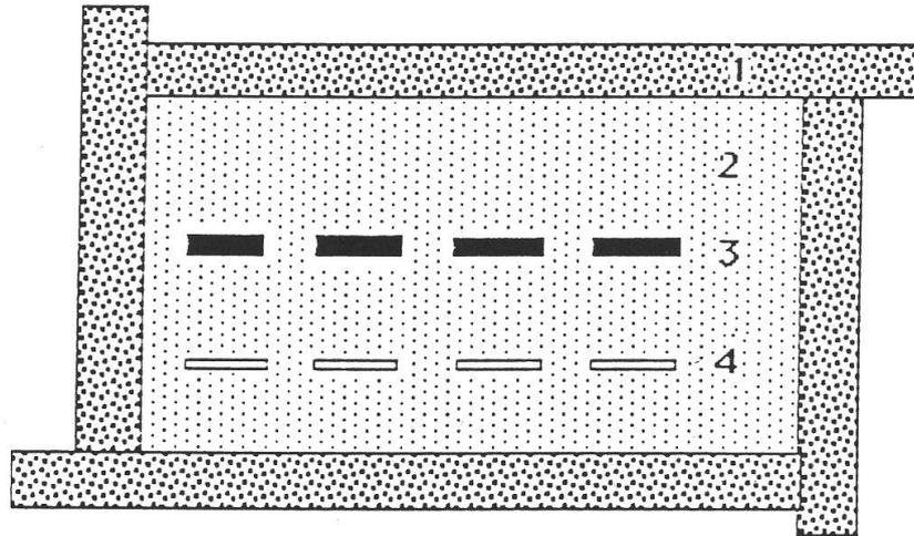
Fig. 3. Scheme of agar overlay. 1) Rubber frame; 2) Agarose gel with agar overlay on top; 3) enzymes (seen due to formazane reaction); 4) Start.
