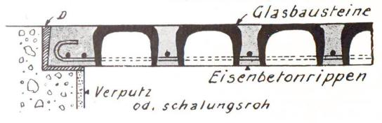
D = joint de dilatation, asphalte ou bitume coulé
