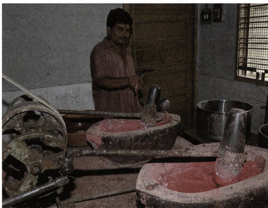
Figure 14: Mechanisation of the long processing procedure, iracam -based formulation. Photo taken at the Government Siddha Medical College GSMC, Palayamkottai ©Christian Sébastia.
