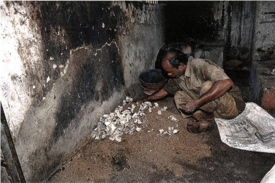
**Figure 17:** Preparing the calcinations of *kasturi karuppu* (method of obtaining a moderate temperature).
