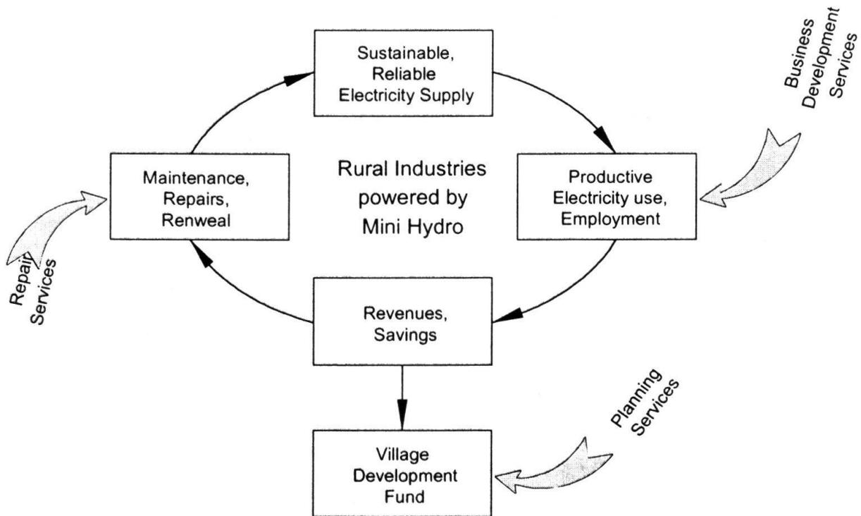
Figure 7: Integration of Mini Hydro Operation and Productive Electricity Use.<sup>19</sup> Above: Current Mini Hydro Development Approach. Below: The SIAM-Approach.
