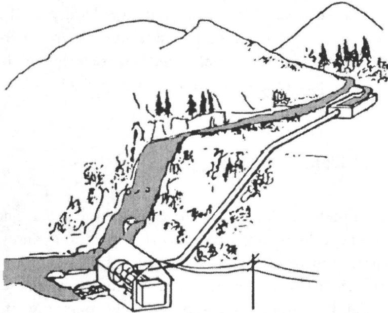
Figure 1: Possible Layout of a Mini Hydro Scheme<sup>3</sup>
