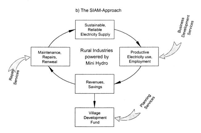
Figure 7: Integration of Mini Hydro Operation and Productive Electricity Use. 19 Above: Current Mini Hydro Development Approach. Below: The SIAM-Approach.
