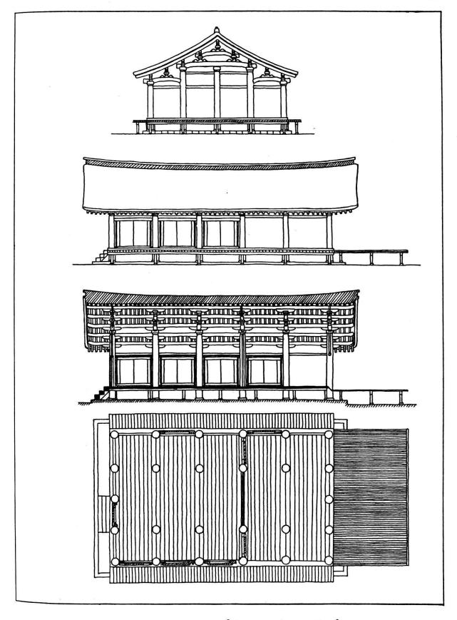
Fig. 3. Tentative reconstruction of the original Dempôdô of Hôryûji
