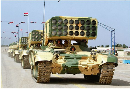
Mobile Raketenwerfer 122 mm TOS-1 «Buratino». Bilder: IRQ Min of Defence)
