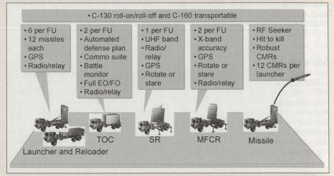
Easily deployed to the conflict, MEADS is designed to keep pace with fast-moving maneuver forces.
