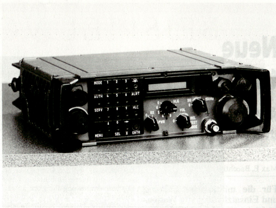
Tragbare 4-Watt-Station PR4G (Poste Radio 4 e Génération)
