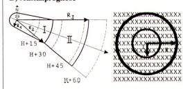
$(R1) = 4.2 \, \text{km}$ Radius NP Radius Zone I  $(R2) = 30 \, \text{km}$ Radius Zone II (R3) = 60 kmWindrichtung = 15 Dekagrad Windgeschwindigkeit = 30 km/h H + 15' = 1559
